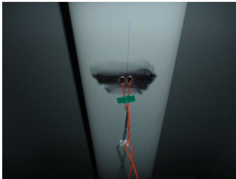
Fig. 11 Installation picture of foil-type strain gauges
