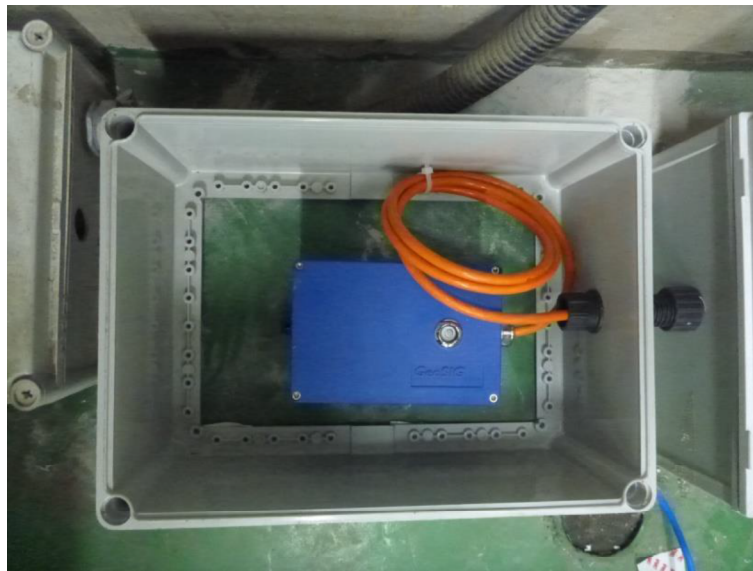
Fig. 10 Installation picture of the seismometer
