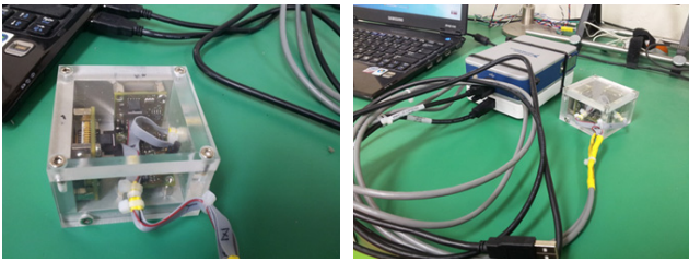
Fig. 5 The sensor module, electric wiring and DAQ board
